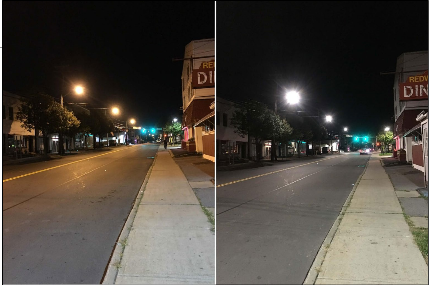
Streetlights before and after LED conversion, East Syracuse
